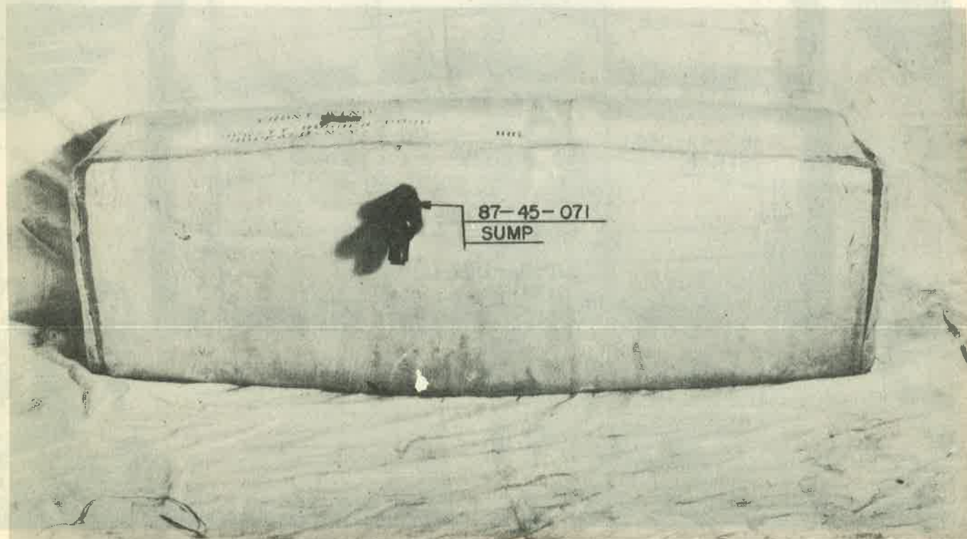
FIG.80 FUEL TANK WING - FRONT H-87A-2 & H-87A-3
