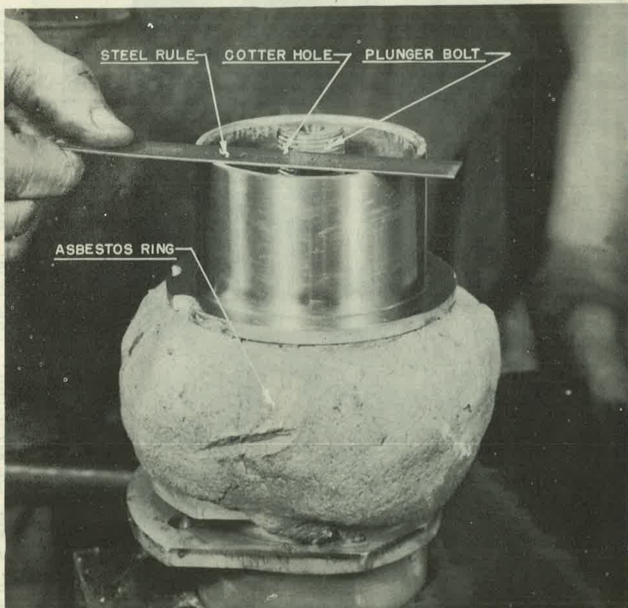
FIG.53C CHECKING COTTER HOLE LOCATION IN PLUNGER
