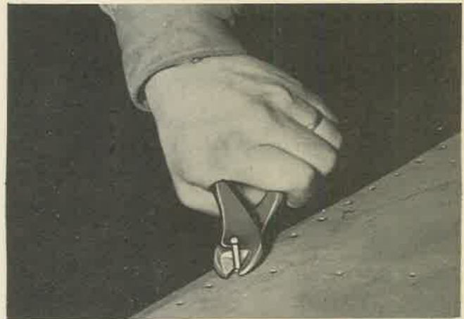
Figure 103—Cherry Rivet Installation
