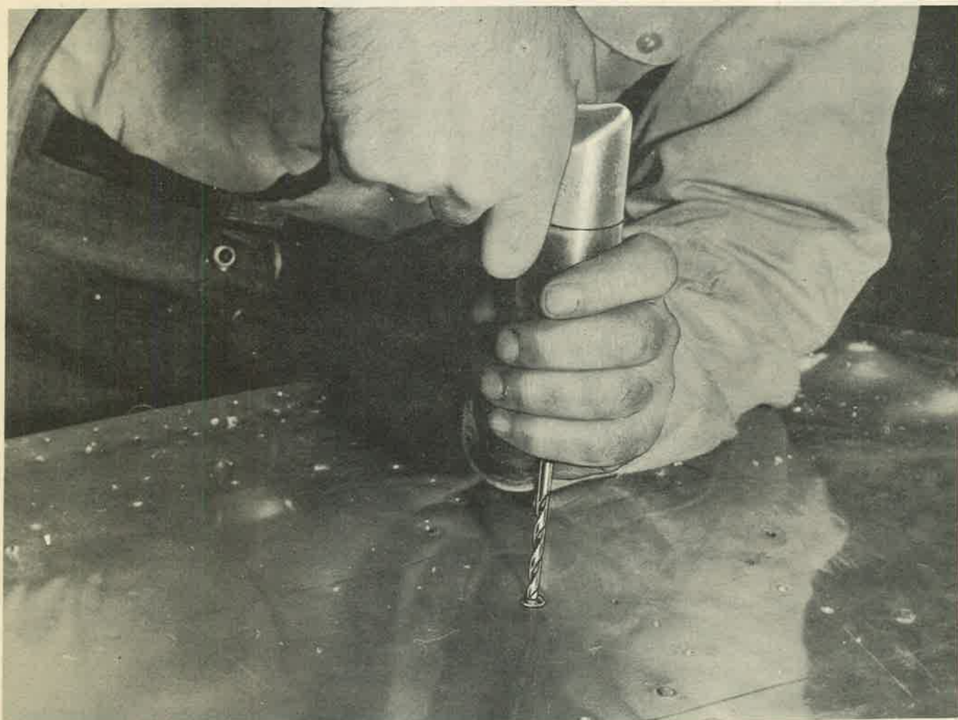
Figure 138—Drilling Rivet Head
