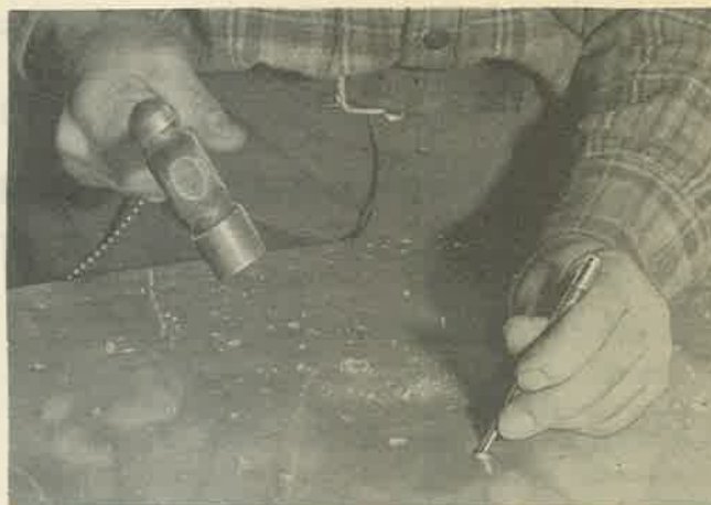
Figure 140—Removing Rivet Head with Punch
