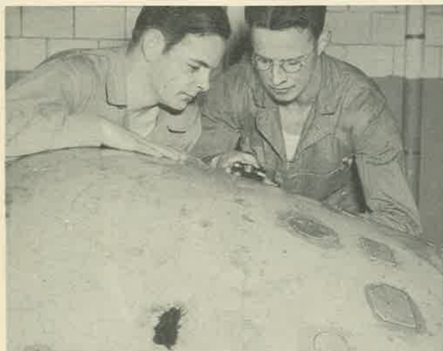
Figure 146—Patching Stressed Skin
