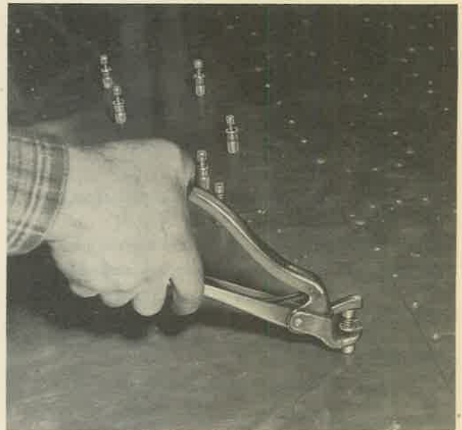
Figure 143—Clamping Panel in Place with Cleco Fasteners
