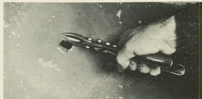
Figure 150—Trimming Out Hole
