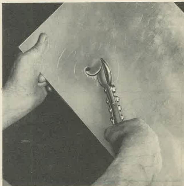
Figure 65—Cutting Inside Curve with Aviation Snips
