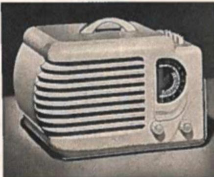
**TABLE MODEL AT-15:** Molded ivory plastic cabinet. 5 tubes, AC-DC superheterodyne circuit, standard broadcast range, push-button tuning, Bilt-In-Tenna, automatic volume control, 5-inch permanent magnet speaker.
