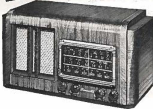
This beautiful AC Table Model, BT-600, is a remarkable value. 110/220 volts, 50/60 cycles, with intermediate transformer taps. 8-inch speaker. 6 tubes. 3-gang condenser. Tuned RF stage. 5-watt output. 3-band set—555 to 13 meters, full coverage on Tropical Band. Phonograph and television jacks. Cabinet dimensions 11 inches high, 22 inches wide, 10½ inches deep.
