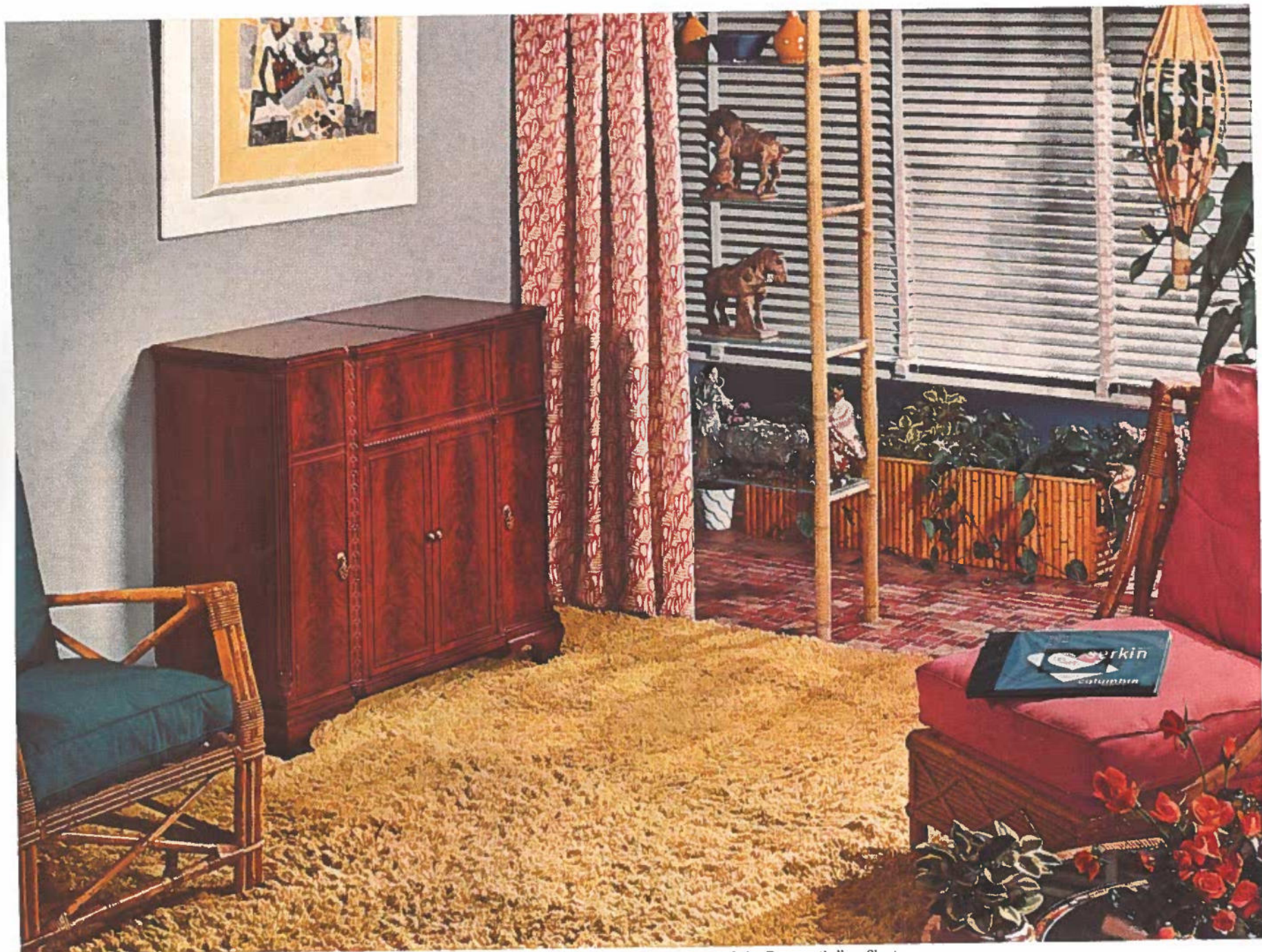
THE FARNSWORTH CHIPPENDALE CONSOLE • Brilliant phonograph-radio in a cabinet of truly regal beauty—proud master of the Farnsworth line. Short-wave, standard and FM (Frequency Modulation) reception. Treble and bass tone controls. Automatic record-changer. Beautifully finished in rich mahogany.
