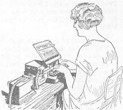
Today messages are sent by an operator seated before a machine that resembles a typewriter as illustrated above. As she types the message on the keyboard the machine automatically punches holes in a tape, each letter having a certain distinct group of holes. This tape, a sample of which is shown below, runs through a transmitter at the side of the sending machine which automatically interprets the holes into electrical impulses that flash over the wire.
