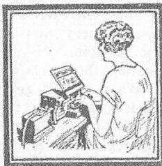
The message has been given to an operator of an automatic machine who prepares the message for transmission, and as she touches the keys of the typewriter-like machine, the telegram speeds to the distant city.
