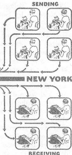
four operators pounding keyboards that perforate tape which is automatically translated into electrical impulses. At each end of this tiny wire there are also four typewriter-like machines called printers that receive these electrical impulses and change them automatically into the proper letters and then type these letters on a blank or paper tape. The receiving operators do nothing but feed the yellow blanks to the machine.
