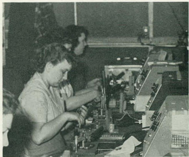
OSCILLOSCOPE CHECKS all reed tuning in electronic piano. Each tuner has individual machine shown below.
